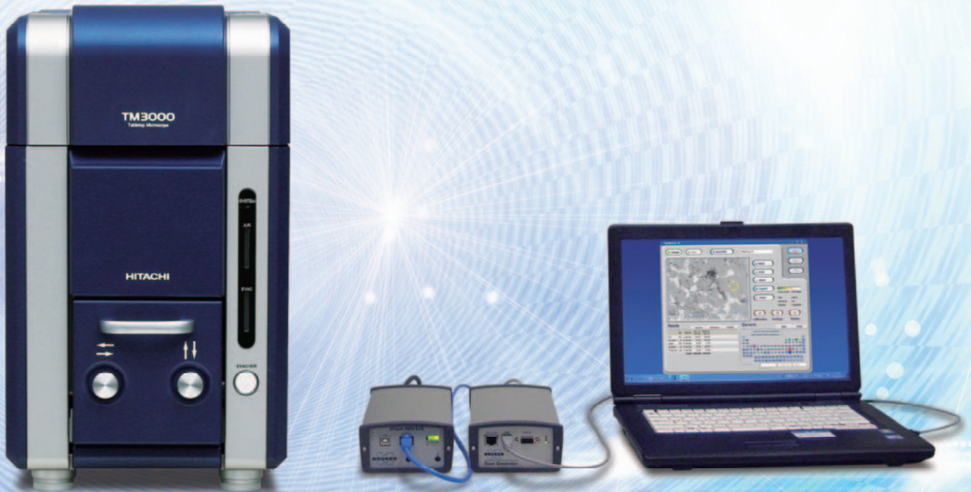
*Typical Configuration of TM3000 with Quantax70 *Built-in EDX detector
